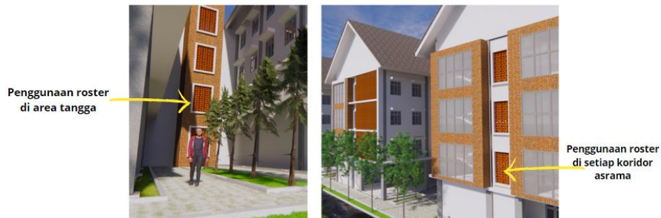
Figure 12. Use of breezeblocks in dormitory buildings
